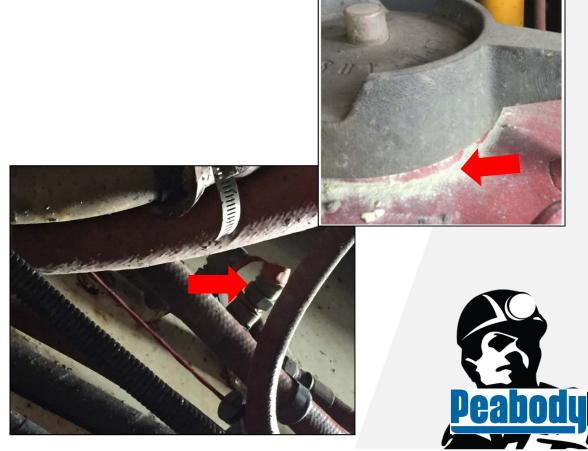
Fire wire for auto activation of the fire suppression system is located below the cable ignition risk by > 1 metre.
