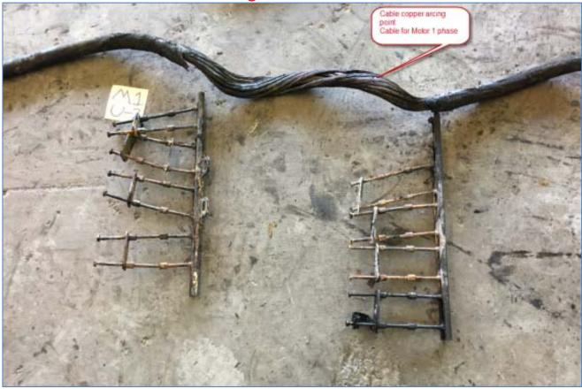
Identified cable arcing on Motor 1 Phase U-2.
