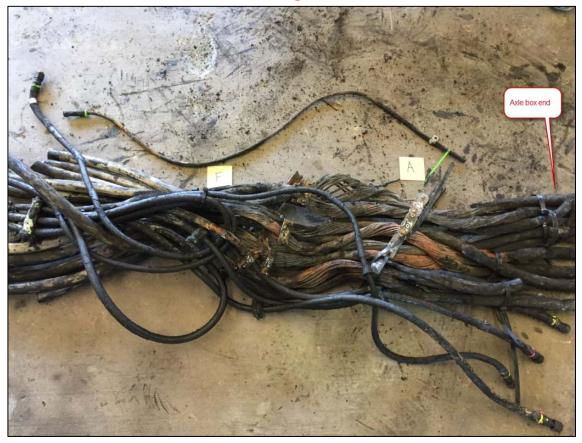
High Voltage harness and hydraulic lines removed and inspected
