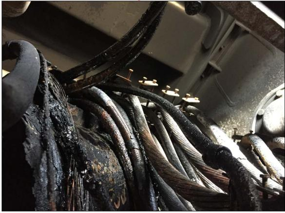
Close up view of the High Voltage harness and hydraulic lines
