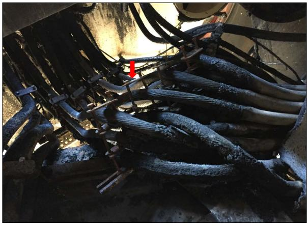
View looking down on the High Voltage harness and hydraulic lines
